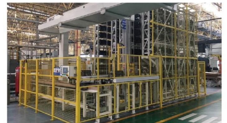
发动机缸体缸盖数字化缓存系统 | Engine block cylinder head digital buffer system
